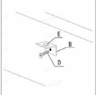
Attach metal angle B to side rails with part D bolts and put on chip E.
