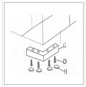
Install legs G to headboard and footboard with D bolts, put part H under the wood leg.
