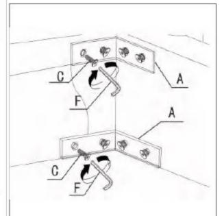
Attach metal angle A to headboard, rails and footboard, using C bolts.
