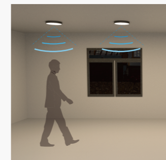
With insufficient ambient light if any motion is detected, all the lights switch on at the same time.
