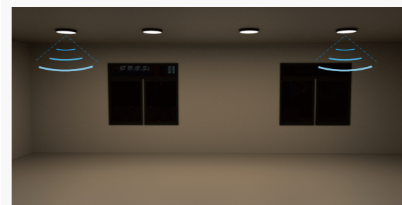
After delay time, the master and slave lights dim to a low light level if no new motion trigger.
