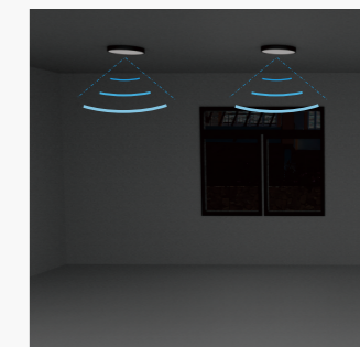
After hold time, the master and slave lights switch off when no new motion trigger.
