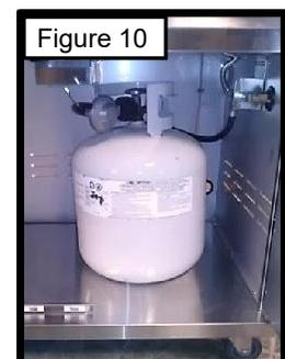
9. Open tank valve SLOWLY (counterclockwise) until fully open. Use a soapy water solution to check all connections for leaks before lighting grill. If a leak is found DO NOT use the grill. Turn gas off and call a professional gas fitter to repair the leak.
