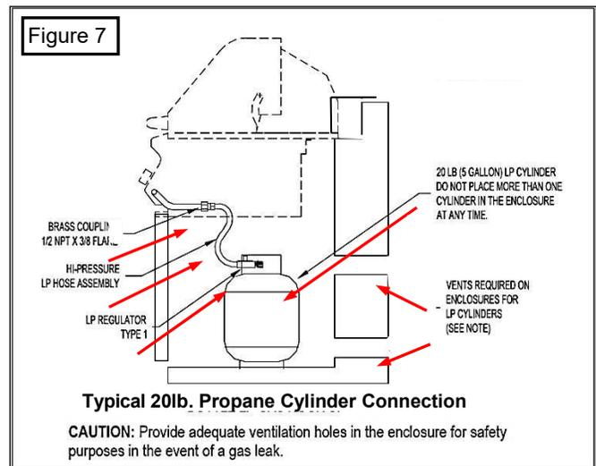
■ **CARTS: INSTALLING & CONNECTING A PROPANE CYLINDER TO THE GRILL:**
