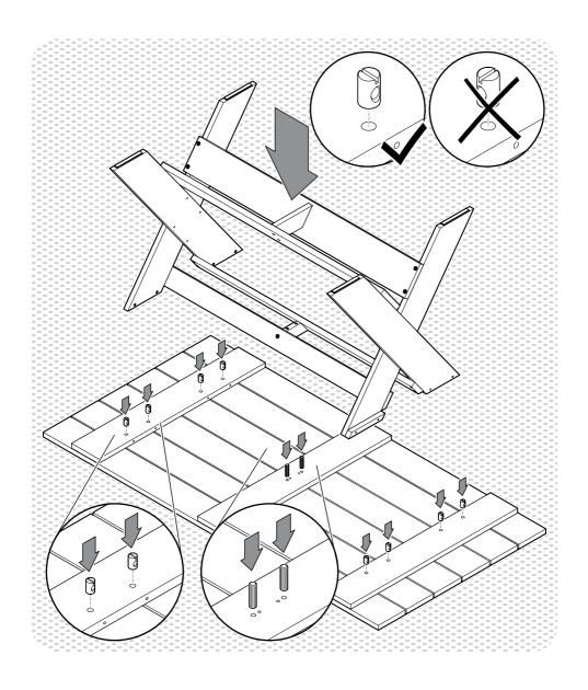
Secure the leg sections to the tabletop using screws ①. Pay attention to the different lengths of screws. First tighten all the screws loosely, before tightening them completely.
