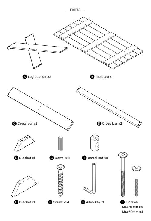
Connect the first cross bar **C** to the leg sections **A**. Make sure the leg sections are positioned as illustrated. Secure with screws **H** and dowels **G** in between. First tighten all the screws loosely, before tightening them completely.
