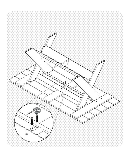
Secure the bracket  $\textcircled{\textbf{B}}$  to the tabletop with screws  $\textcircled{\textbf{H}}$  .
