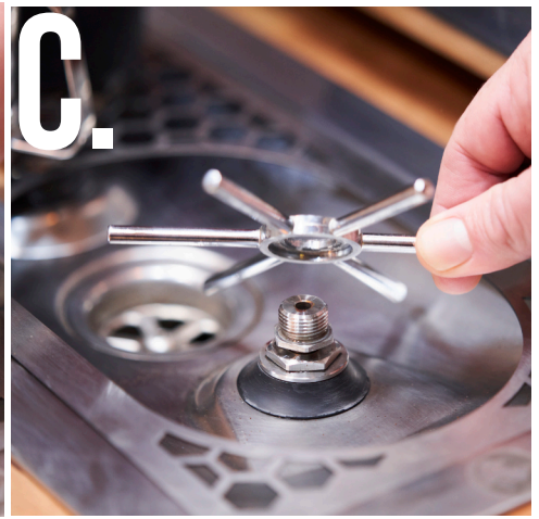
(C) Remove the actuator star by lifting it over the top of the valve
