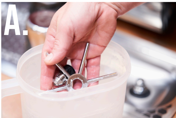
(A) Immerse the Spinjet and actuator star in the cleaning solution for 10 mins.
