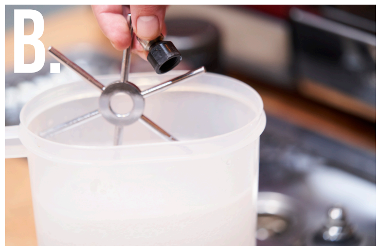
(B) After 10 minutes, remove the Spinjet tip and actuator star from cleaning solution and rinse thoroughly with clean water.
