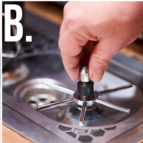
(B) Replace the Spinjet by attaching to the spray valve.
