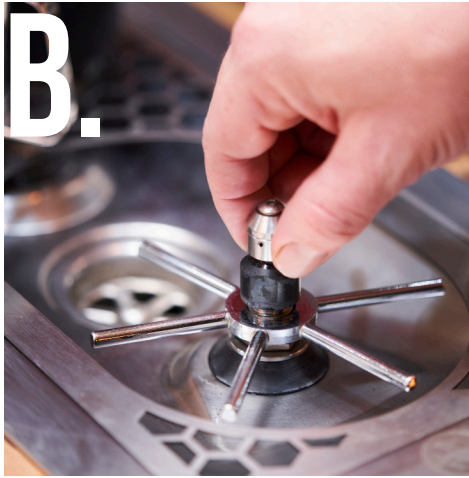
(B) While holding the actuator star in place, unscrew the Spinjet from the spray valve. (Be careful not to rotate or spin the actuator.)
