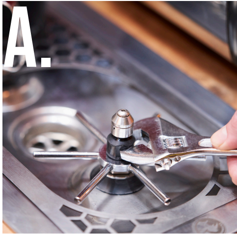
(A) Using an adjustable wrench, locate the 2 notches at the base of the spinjet
