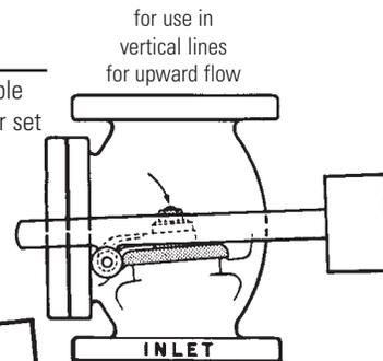
The lever and weight is mounted on the right side of the valve when facing the inlet. Available on Figure no. F-918 in sizes 2½"–12".
