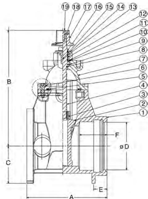
Coating — Electrostatically applied fusion-bonded epoxy 8-20 mil. inside and outside.
