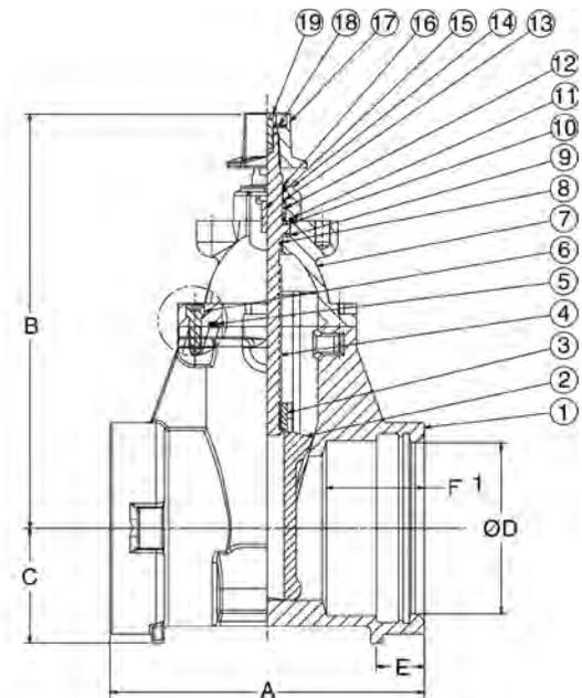
**Coating** — Electrostatically applied fusion-bonded epoxy 8-20 mil. inside and outside. Meets or exceeds performance requirements of AWWA C550. Epoxy coating is not intended to serve as a dielectric barrier internal to the piping system.
