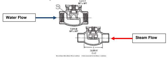
After the valve has been installed, the valve should be tested to make sure that it opens and closes easily and that the bonnet joints or pipe joints are not leaking.
