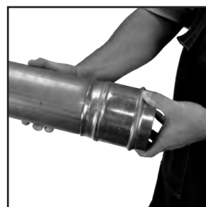
Figure 9: Inspection of final crimp
