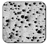
Ductile Iron Spheroidal Graphite Nodules
