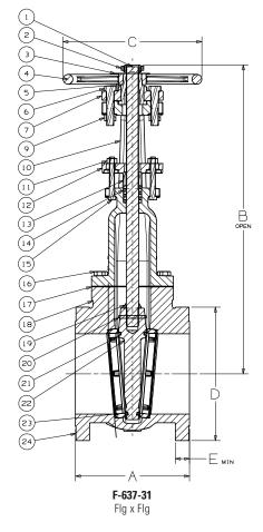
FREEZING WEATHER PRECAUTION: Subsequent to testing a piping system, valves should be left in an open position to allow complete drainage.
