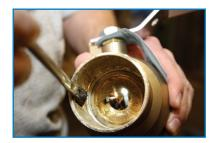
**Heat:** Silicon bronze alloys will transfer heat away from the heat affected area more slowly than copper or leaded bronze; therefore, more attention may be required to achieve uniform heating of the alloy. Select torch tip and gas mix to adequately distribute the heat. The hotter the flame, the more skill and technique are required.
