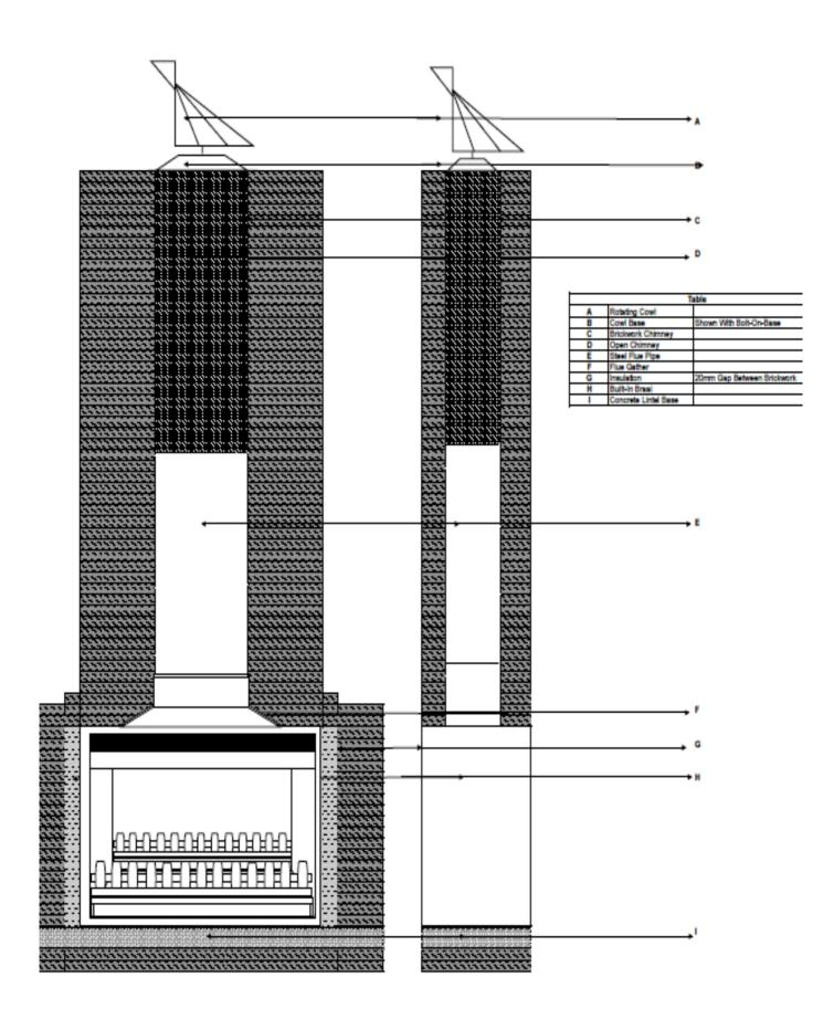
Fig.1 Typical installation of a Megamaster Built-In Fireplace
