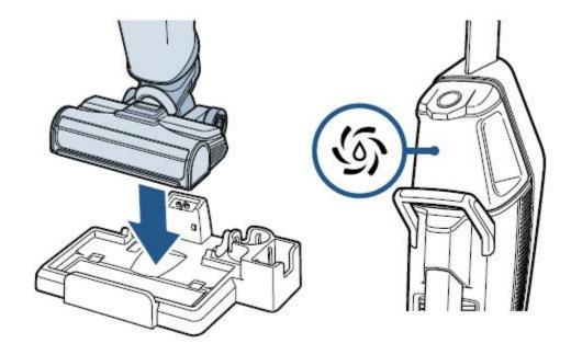
Press clean out cycle button and let machine go through full 40 second cycle
