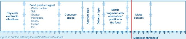
Figure 7. Factors affecting the metal detection threshold.
