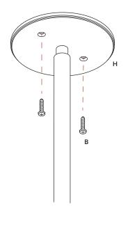
**Step 6:** Gently slide the canopy cover back up the stem (H). Rotate the canopy cover clockwise to secure firmly in place.
