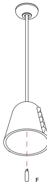
**Step 9:** Thread the diffuser over the bulb (D). Turn the power back on at the main fuse box or circuit panel you disabled before installation.
