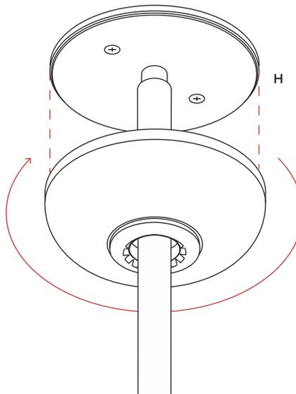
**Step 7:** Carefully align the socket with the hole in the shade, and slide the shade up. With one person holding the shade (G) in place, use the included tool (E) to thread the washer, tightening the shade to the stem (H).
