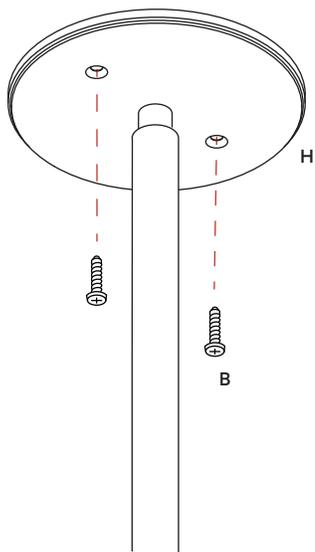
**Step 6:** Gently slide the canopy cover back up the stem (H). Rotate the canopy cover clockwise to secure firmly in place.
