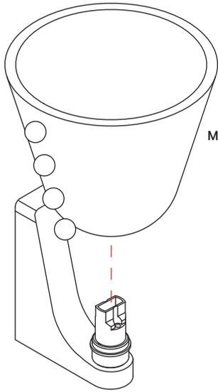
**Step 10:** Secure the shade (M) into place using the washer and provided tool (H).
