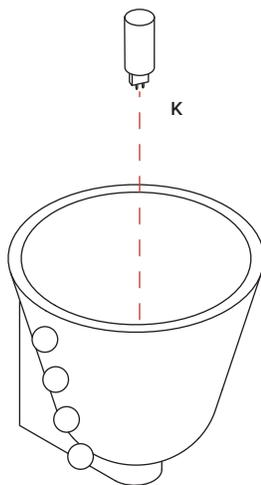
**Step 12:** Thread the diffuser (L) over the bulb. Turn the power back on at the main fuse box or circuit panel you disabled before installation.
