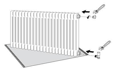
Apply PTFE tape to valves and screw into bottom of radiator tighten with a spanner.
