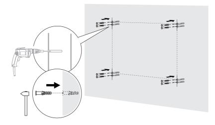
3 Fix the wall brackets to the wall with screws provided and ensure a secure holding.
