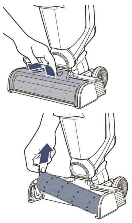
Check ends of brush roll for wrapped debris or hair
