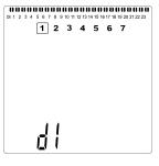
• Use the "+" or "-" keys to select one of the preset programs, d1 to d9 (picture 6), or one of the user definable programs, U1 to U4. The program number will blink. The heating schedule for the current day is displayed along the top of the LCD screen.
