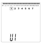
Use the "+" or "-" keys to select a user definable program, U1 to U4, to be modified, then press and hold the "OK" key for 3 seconds.
