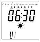
Press the "OK" key to confirm the time at which the mode will change over from Reduced to Comfort. The \* symbol will start to blink instead of the symbol, signifying the start of this Comfort period.
