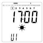
Press the "OK" key to confirm the time at which the mode will change over from Reduced to Comfort. The \* symbol will start to blink instead of the symbol, signifying the start of this Comfort period.
