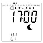
Use the "+" and "-" keys to adjust the time at which this Reduced period will end.
