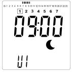
Press the "OK" key to confirm the time at which the mode will change over from Comfort to Reduced. The Symbol will start to blink instead of the \* symbol, signifying the start of this Reduced period.
