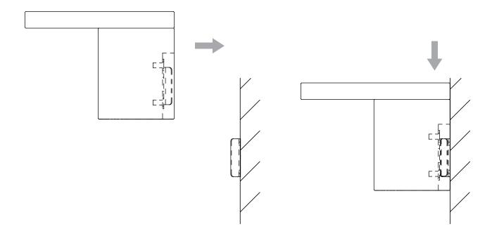
NOTE! Load weight should be distributed evenly and with a maximum weight of 5kg for the 80 cm shelf and 8kg for the 120 cm shelf
