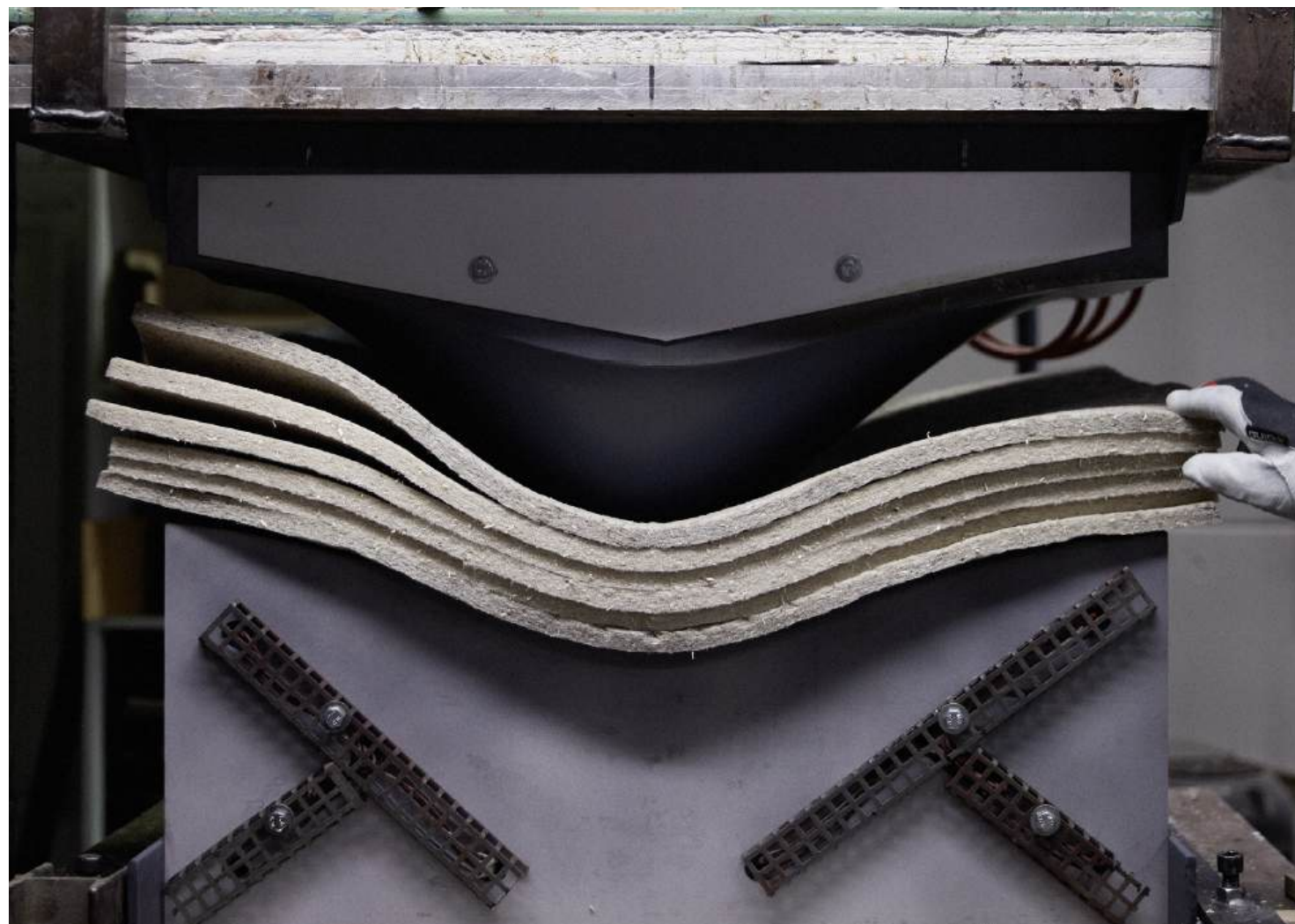
Mat Chair shell in the compression process
