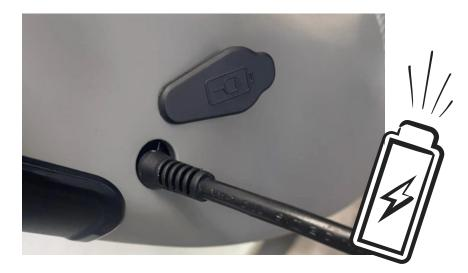
When the battery is fully charged (green light on charger), remove the charger and install the battery into the bike or cover the charging port if left on the bike.
