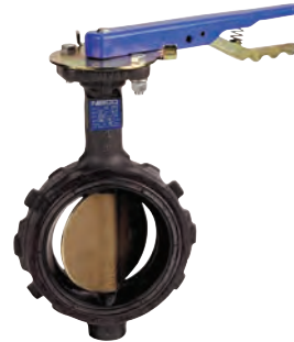
WD-3100 Wafer Style Buna-N Liner and Aluminum Bronze Disc
