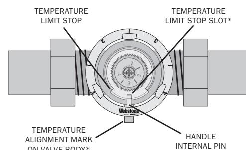
If desired, the temperature setting can be fixed on the Webstone TMV by locking the handle in place:
