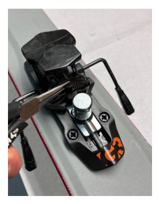
3. Next the brake spring pivot pin(3) will be removed by using the punch pin as a guide to punch the pivot pin(3) out with a hammer. The pivot pin is directional and will only come out one way, if you are looking along the ski towards the tip the pin will come out to the right, see photos below. Once the pin has been punched out enough to expose the knurls on the other end pull the rest out with pliers.
