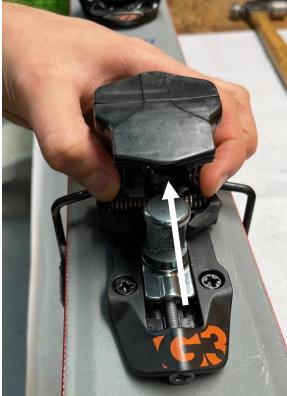
5. Flip the brake over to expose the 4 torx screws(4)(5) and use a T10 or 7/64"driver or allen key to remove them and place them aside for later. The two screws in the top of the photo that are wider apart are shorter than the bottom two that are close together.
