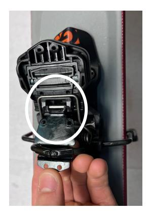
7. While holding the brake platform cover(11) and brake platform(8) together rotate the brake arms until they are parallel with the ski and use vise-grips to hold them together while you place the screws back into their correct spots detailed in step 5, see photo below. Take care not to cross thread the inserts.
