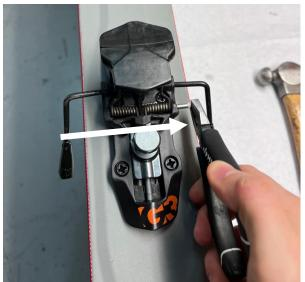
4. To free the brake torsion spring(2) from the brake base(1) place the brake arms perpendicular to the ski as shown in the photos below. Then pull/push the brake torsion spring(2) towards the front of the ski, the two prongs of the spring should pop out relatively easy.
