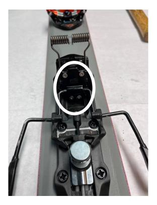
6. Remove the broken or faulty spring from the brake platform cover(11) and replace with the new one in the same orientation as before. The brake torsion spring(2) and brake arms will fit neatly into slots underneath the brake platform(8) and brake platform cover(11) respectively, see photos below.
