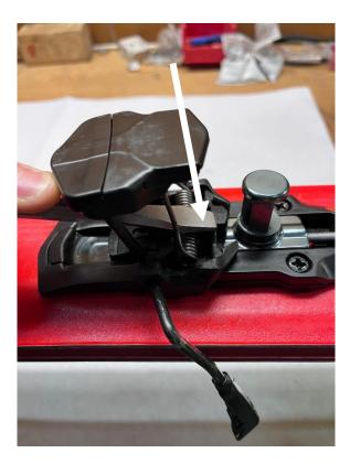
9. Place brake pivot pin(3) back into place, it should fit easily into one of the holes in brake base(1) when it's in the correct direction and can be secured into place with a hammer until both ends of the pin are flush with the sides of the brake base(1).
