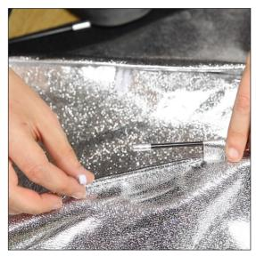
Take one of the rods, and feed the smaller end through the one of the guide-loops located along the internal seam of the softbox backing material.
