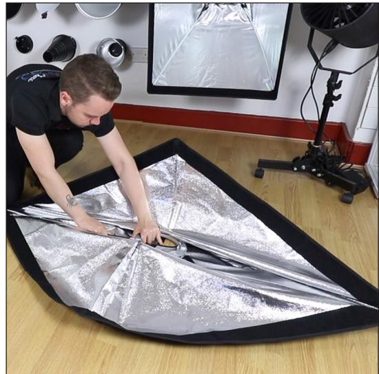
Once the first rod has been inserted, insert the second rod, diagonally opposite the first, and the same process as before.
