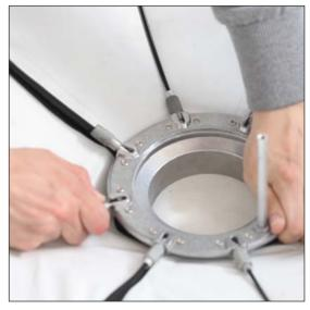
To disassemble the Beauty Dish, simply press down on each of the rods with the heel of your palm, and use your thumb and index finger to release the locks.
