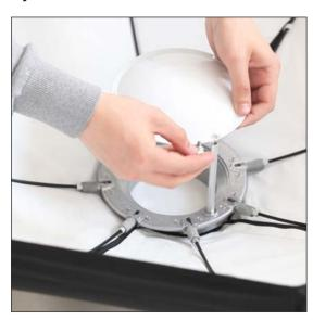
Once the Beauty dish is fully opened up, attach the Deflector, which simply screws onto the top of the spacer rod with a small thumb-screw.
