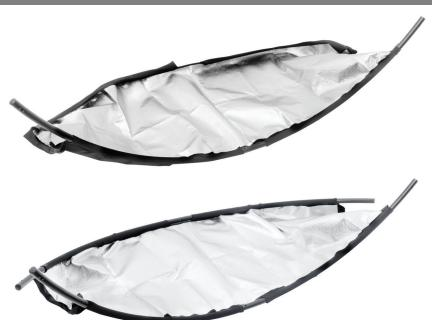
Now that Poles A and B are now all connected together, now feed the pole through the fabric on the long side of the reflector fabric (with the pole curving upwards, and the black side of the fabric facing downwards as shown.
