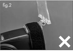
Please ensure that you slide the gel in on the side of the Flip-Gel holder facing away from the speedlite. Sliding the gel in on the side facing towards the speedlite may put the gel at risk of melting.
