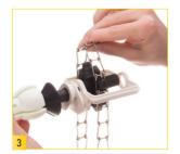
Load the chain onto the gear.
