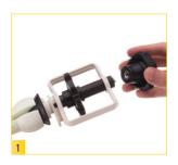
Unscrew and remove the chain drive control knob.
