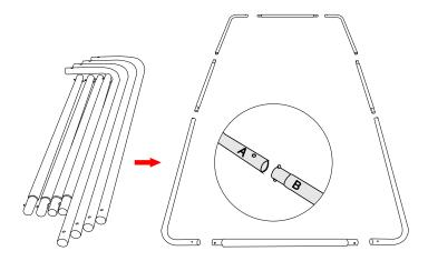
**1** Each frame is combined by 4pcs straight tubes-A and 4pcs curved stubes-B. (As picture).
