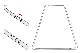
2 Please connnect tube A with tube B by pressing down the spring pin,until it is bounced back.
