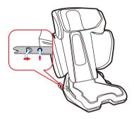
Pull the ISOFIX attachment handle outward and push the seat inward at the same time. For each step forward of ISOFIX attachment, the chair angle will automatically advance one step outward.
