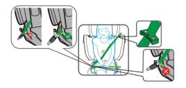
Thread the vehicle seat belt through the shoulder guide hook and the waist belt guide on the child car seat. Place the child in the seat and fasten the vehicle seat belt with an audible click. Tighten the seat belt, and make sure it's not twisted.
