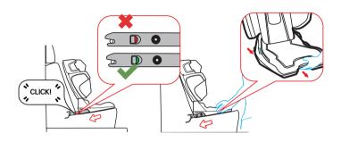
Push the ISOFIX attachment interface on the seat into the ISOFIX attachment anchor point on the car seat until you hear two "click" sounds (please check the red and green indicator on ISOFIX attachment are green to indicate correct installation). Then pull the ISOFIX attachment handle and push the seat inward.
