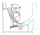
Pull the ISOFIX attachment adjustment handle outward and push the seat inward at the same time. For each step forward of ISOFIX attachment, the chair angle will automatically advance one step outward.
