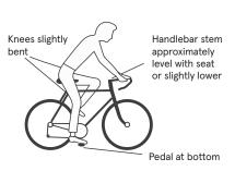
Loosen saddle from seat pillar to adjust forwards or backwards. Tighten when set correctly
