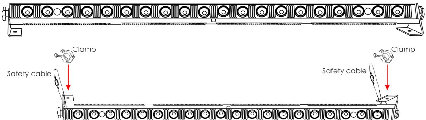
The Sunstrip II Stageblinder can be placed on a flat stage floor or mounted to any kind of truss with a clamp.
