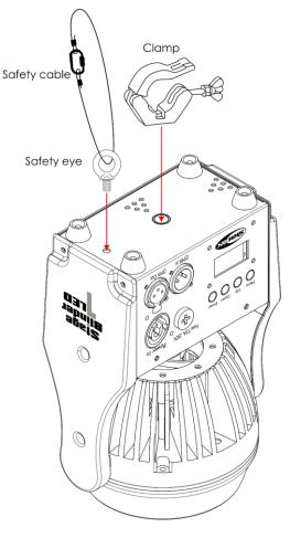
The Stage Blinder 1 LED can be placed on a flat surface or fitted to any kind of truss with a clamp.
