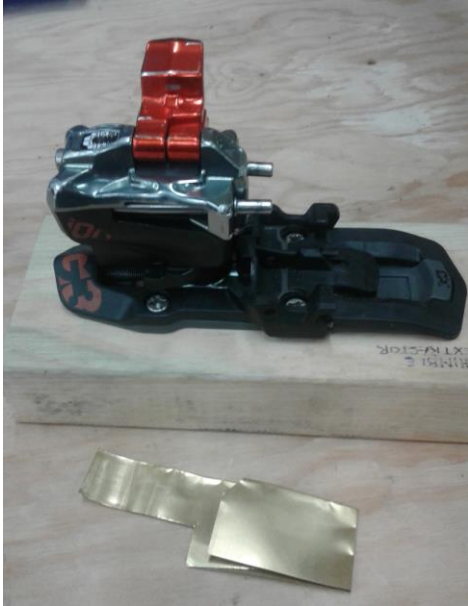
Figure 4 – 0.2mm shim and heel turret.
