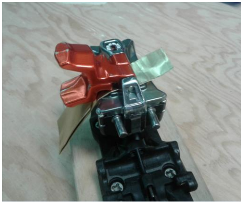
Figure 5 – shim placed under heel lifts
