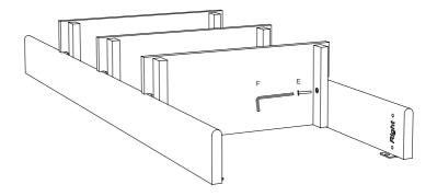
Hold the shelving unit in place where it is to be mounted. Place a spirit level on a shelf to ensure it is straight. Use a pencil to mark through the holes in the hinges where to drill on the wall.
