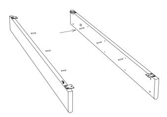
Turn the side rails so the hinges face down towards the ground. IMPORTANT NOTE: Be aware that the marking "right" on the side panel is positioned downward to the right where the bottom shelf is to be attached to the panel, and that the marking "left" on the other side panel is positioned downward to the left. Then slide the three middle shelves between the side rails, ensuring the dowels fits into the slots on the shelf.
