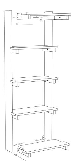
Secure the shelves to the side rails by screwing the short screws (E) through the holes in the shelves and into the side rails using the allen key (F).
