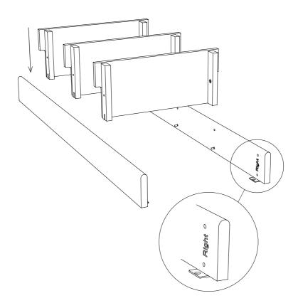
Secure the shelves to the side rails by screwing the short screws (E) through the hole in the shelves and into the side rails using the allen key (F).
