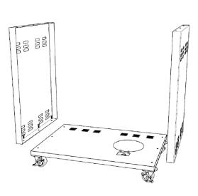
5. Attach Bottom Back Panel - The bottom back panel first gets secured to the Bottom Cart Panel with screws (The bottom of the panel has openings for screws to go through, see diagram). The amount of screws used vary by the size of the grill cart you are assembling. **Attach but to not tighten**. Next secure the Bottom Back Panel to the right and left side panels. Three screws get used per side. **Attach but do not tighten**.
