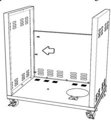
6. Attach Upper Back Panel - This panel gets attached to the left and right panel with 2 screws per side. Attach but do not tighten. Attach the Tank Interference Bracket - (Not included for a 3 burner cart model). This pieces are to intended interfere with a second LP tank being stored inside the grill cart which is not permitted. Using 4 screws, attach and tighten the Tank Interference bracket to the 4 nutserts adjacent to the large circular cutout for the LP tank (see figure D)
