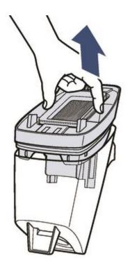
• Hand wash filter & screen with warm water, remove debris
