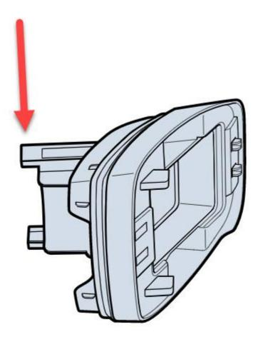
Wipe gold sensors on top of dirty water tank lid below the filter with a dry tissue
