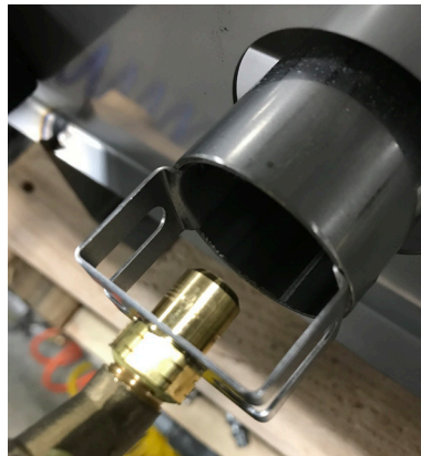
HEARTH BURNER PROPERLY SEATED
