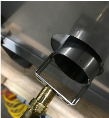
HEARTH BURNER NOT PROPERLY SEATED
