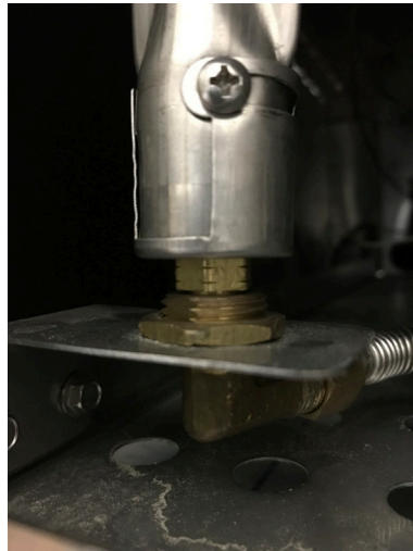
REAR BURNER PROPERLY SEATED
