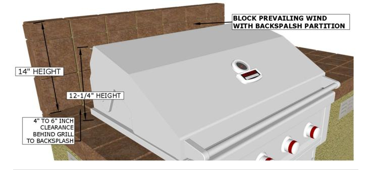
**<u>ATTENTION</u>**: Take special precaution when installing grill in open Breezy area, check the direction of Prevailing Wind Direction, if back of grill is facing any oncoming wind or breeze, be sure to protect the back of grill, and erect a partition wall, or only use grill with hood open on breezy days.
