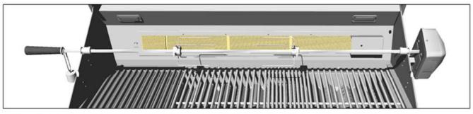
INSTALL DOUBLE POSITIONS IN BOTH HIGH & LOW POSITION, MOUNT MOTORS CRISS-CROSS FROM EACH OTHER, DO NOT USE ROT. ROD WEIGHT.
