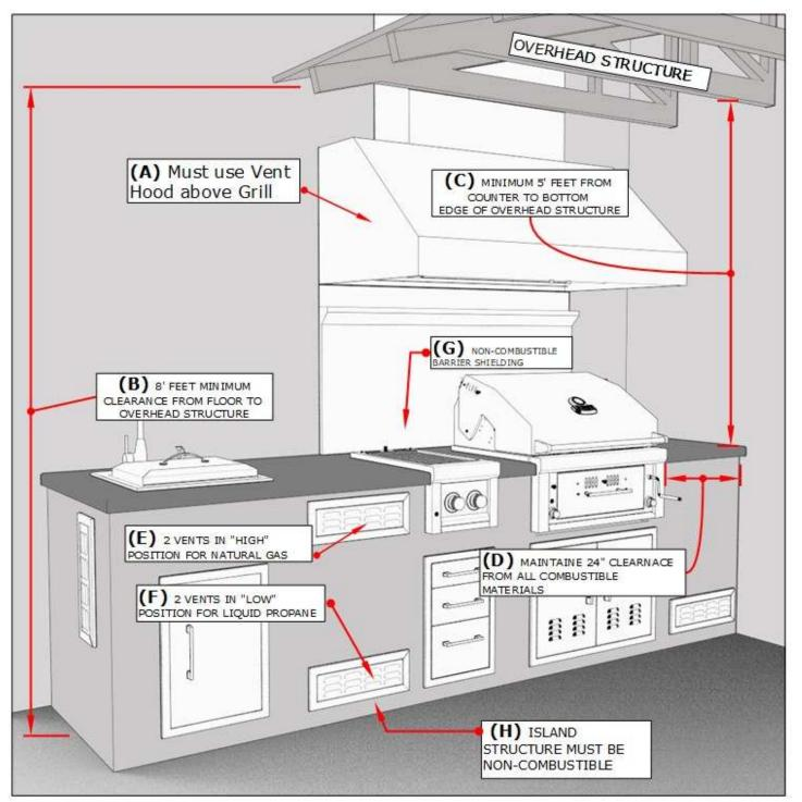
**ATTENTION:** All Gas Grill Installations MUST HAVE MINIMUM TWO AIR-FLOW VENTS, either in ELEVATED POSITION for Natural Gas or LOWERED POSITION for Liquid Propane. Your Warranty may be VOID if island does not meet basic setup requirements.
