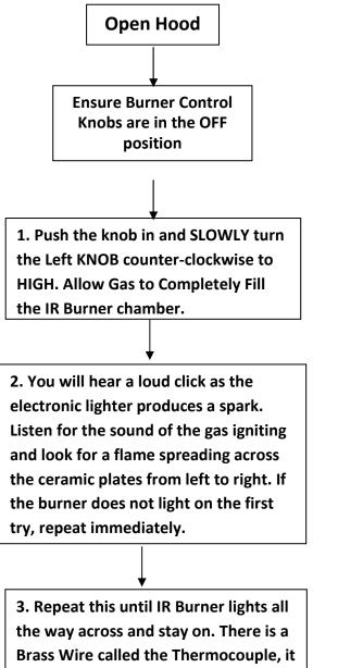
TIP: If IR-Burner does not stay lit, try running the bottom burners first for 10-15 minutes, this will heat the Thermocouple and help the IR-Burner stay lit.
