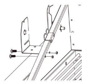
through the bracket. Place a washer on the end of each bolt. Secure bolts with nuts. Take care not to over tighten the bolts. The slide the rotisserie motor onto the bracket.
