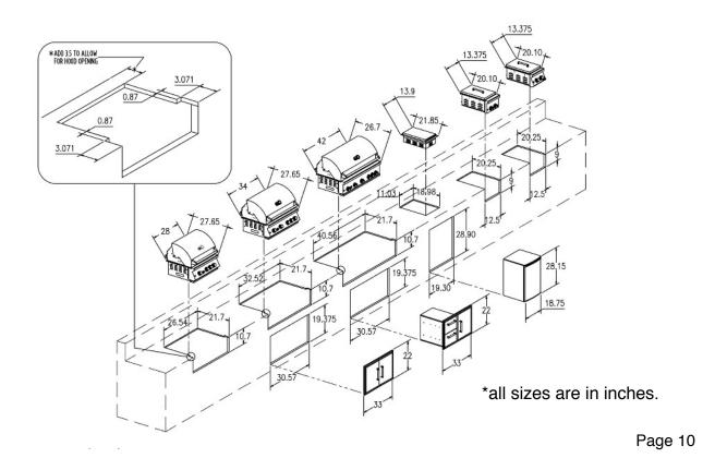
Your choice of masonry can be used for cabinet construction for the built-in gas grill; however it must be **non-combustible** material. Keep in mind when choosing a location for your grill that it should **NOT** be located under any overhead combustible construction.
