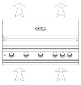
Proper airflow MUST be maintained for the grill to perform as it was designed. If airflow is blocked, overheating or poor combustion will result. Do not block the 1" (2.5 cm) front air inlet along the bottom of the control panel or more than 75% of the cooking grid surface with pans or griddles.
