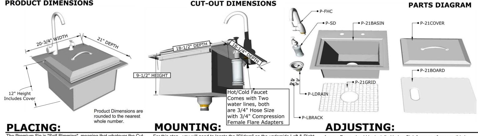
The Premium Sin is "Self-Rimming", meaning that whatever the Cut-Out edge looks like, as it is always rough, the product rim will cover all edges. Make the Cut-Out in counter surface matching to our provided dimensions shown, and simply insert Sink in through the open hole. It will Free-Hang so do not build any support below it, all other mounting brackets are included.
