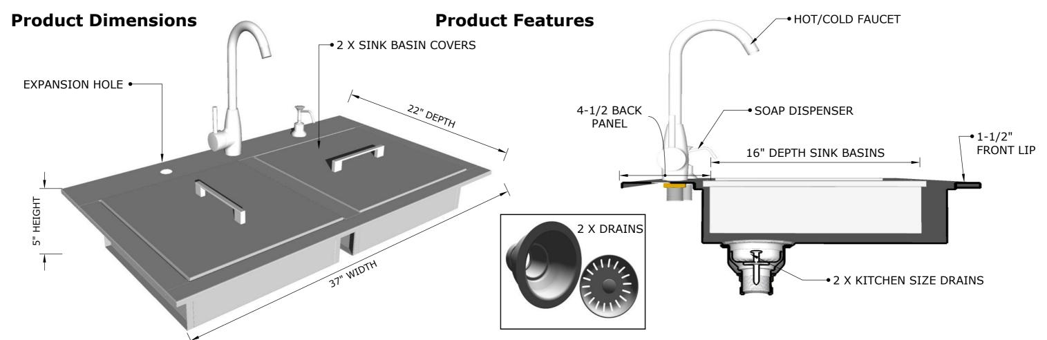
DROP-IN COUNTER CUT-OUT SIZE IS 35" WIDTH BY 3-3/4" HEIGHT BY 19-1/2" DEPTH
