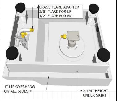
WARNING: Never build shelf or enclose interior space under the Burner Cut-Out. The Side Burner is Self-Rimming and is supported by the top counter. The bottom of Burner needs to be open to allow for proper ventilation. ALLOW 6 INCH MINIMUM CLEARANCE FROM UNDERSIDE OF COUNTER BURNER BACK TO INTERIOR ISLAND WALL — MUST ALLOW AIR FLOW AROUND BACK OF BURNER.
