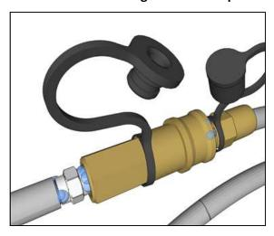
**Test connection from burner to LP Hose**
