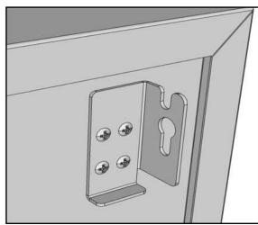
WHEN INSERTING EACH WING, PUSH PINS INTO ADJACENT BRACKETS AND PUSH PINS ALL THE WAY OVER ALLOWING OTHER SIDE TO SLIDE ALL THE WAY INWARD, HINGING PINS THROUGH SOCKET HOLES THEN SLIDING WING CENTERED MOUNTING WING.
