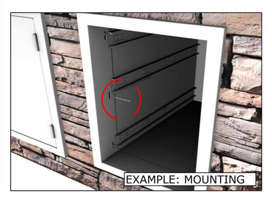
Check the Alignment of the Drawer Box that is Horizontal, add additional Shimming in back of box if needed. If you have not already installed the Handles - Please do that now, handles come packaged pinned inside the drawer face, you may need to reverse them using a Screw Driver. If any individual drawer faces are uneven, see the Left/Right Two Screws of Drawer Face Panel connecting to box. Loosen either the Top or Bottom Screw on the Left/Right Side making adjustments in the drawer face pane.
