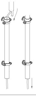
Pull precisely and with caution at the power cord to ensure a tight fitting of the two lamp parts
